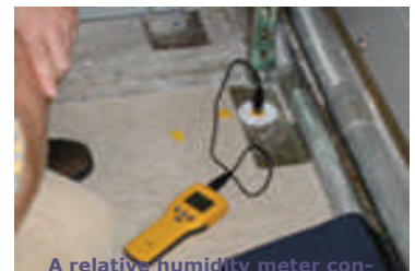
A relative humidity meter connected to the probe yields an internal moisture reading. Relative humidity testing represents advanced concrete moisture testing for the 21st century.
