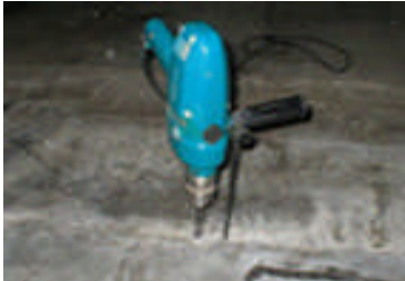
By drilling a hole in the concrete, the F2170 method can measure moisture deep inside the slab.
